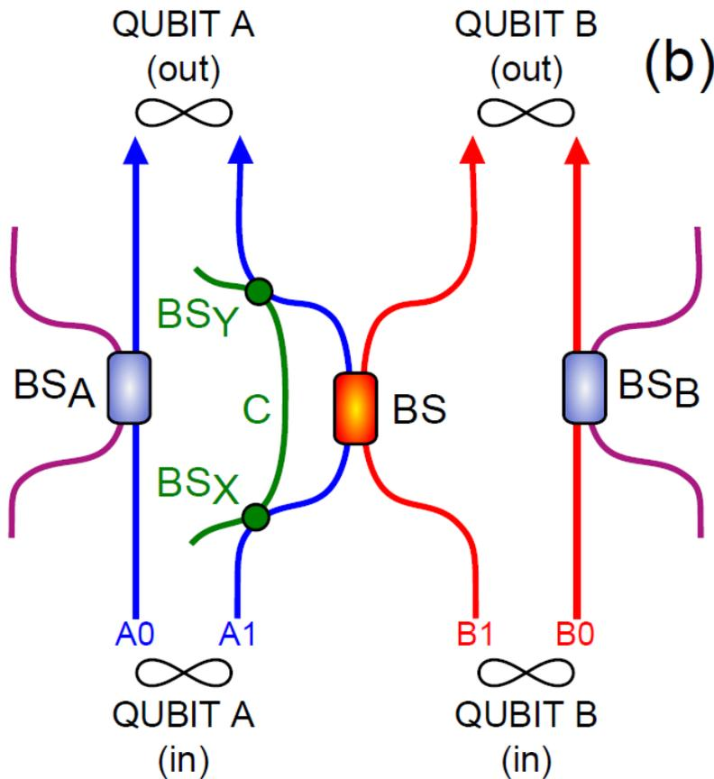
Mode A1 is coupled to auxiliary mode C
