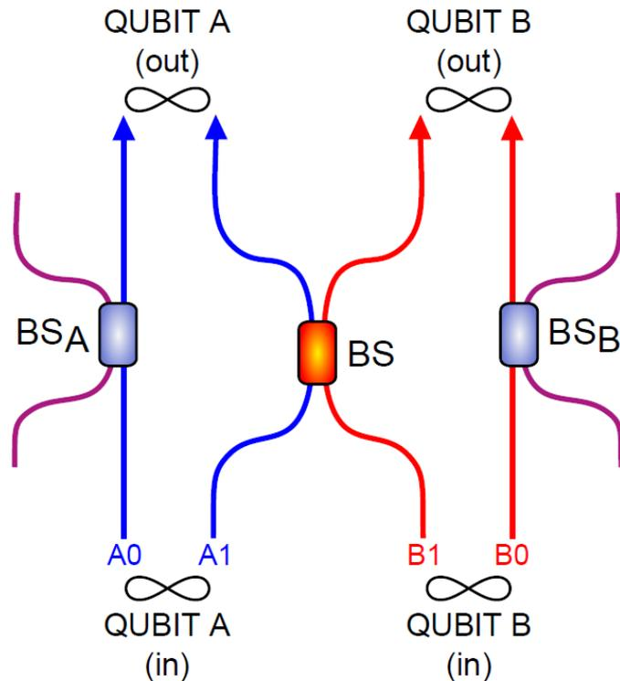
The three beam splitters  $BS$ ,  $BS_A$ , and  $BS_B$  are identical.
