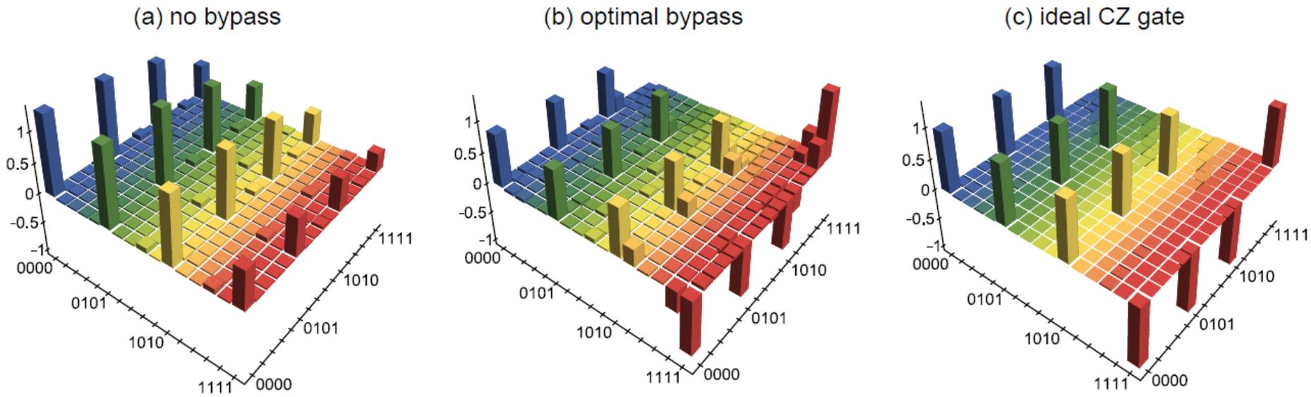
FIG. 5. (Color online) Quantum process tomography of the CZ gate. Reconstructed quantum process matrices  $\chi$  of two-qubit operation without bypass (a) and with optimal bypass (b). For comparison, the ideal CZ gate is shown in panel (c). For ease of comparison, all process matrices are normalized so that  $\text{Tr}[\chi] = 4$ . Experimentally determined success probability of the CZ gate shown in panel (b) reads  $P_S = 1.15(2)\%$ .
