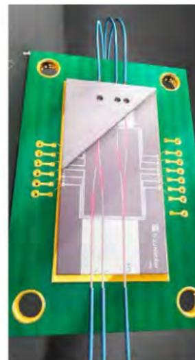
F. Costache et al., Variable optical power splitter with field-induced waveguides in liquid crystals, OFC.2014.Th1A.7 (2014)
