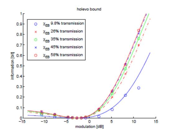
Experimental results, confirming canceling of information leakage at proper modulation at the different values of channel transmittance. Eve's information is directly measured at the output of the channel.
