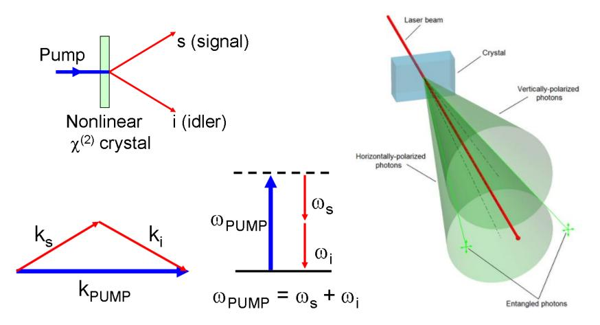
Typical CV entangled states – *twin beams* a.k.a. *two-mode squeezed vacuum states* (TMSV)
