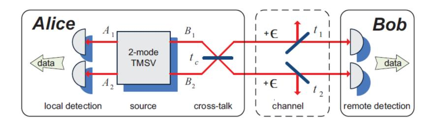
Two-mode entanglement distribution scheme over noisy and lossy quantum channel with cross-talk in the source. Covariance matrix of the resulting state:
