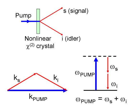
Typical CV entangled states – *twin beams* a.k.a. *two-mode squeezed vacuum states* (TMSV)
