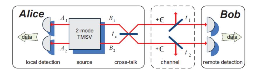
Two-mode entanglement distribution scheme over noisy and lossy quantum channel with cross-talk in the source
