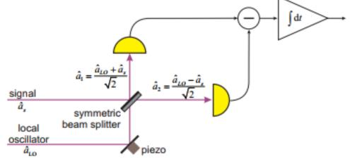
Depending on the phase-shift of the *local oscillator*, x or p quadrature is measured:  $\hat{X}_{\theta} = \hat{X} \cos \theta + \hat{P} \sin \theta$
