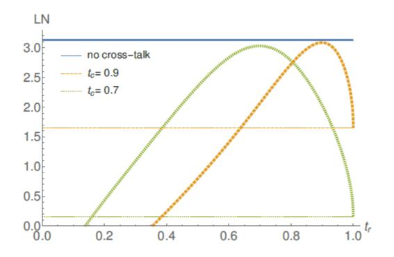
Possibility to restore entanglement in the case of unbalanced channels (transmittance of 0.9 and 0.7 for different modes)
